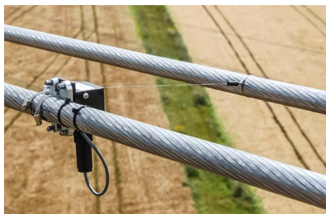
PT1 sensor for sub span oscillation measurement
