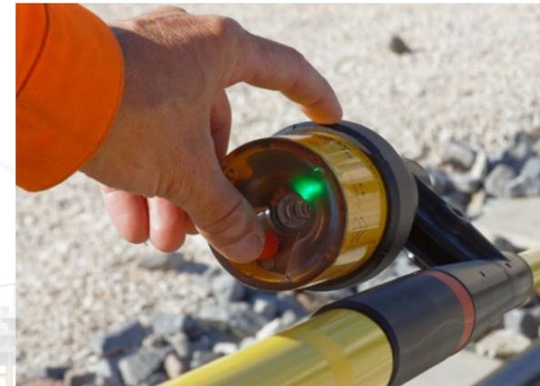
Direct feedback from the voltage detector with active switch-on
