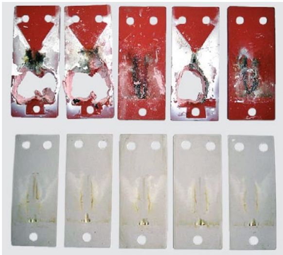
Fig. 9: Erosion resistance of inappropriate filled (top array) and well-balanced (bottom array) Silicone Rubber
