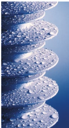
Fig. 10.1: Hydrophobicity of an unpolluted Silicone Rubber surface
