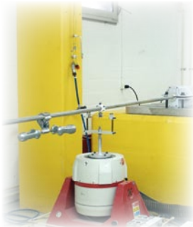
Test Set-Up for Damper Testing
