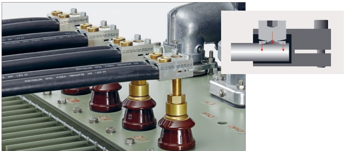
Figure 3: Bolted terminals with spring elements compensate flow and settling processes, such as this 2DIREKT transformer terminal clamps
