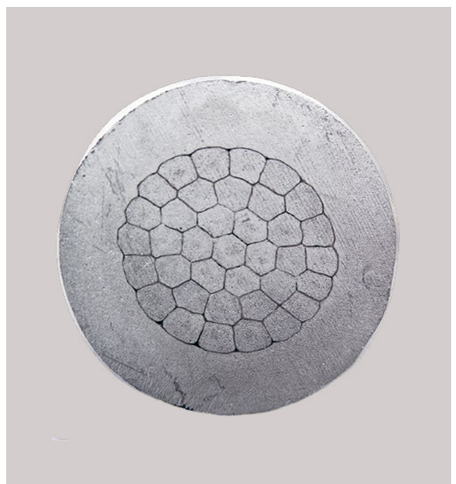
Figure 2: Contacts with long-term reliability require optimal transverse conductivity in the conductor. To achieve this, not only the exterior layers of the conductor assembly when crimping, but also its interior layers. This image shows optimal crimping via symmetric crimping: All individual wires show the characteristic angular distortion.
