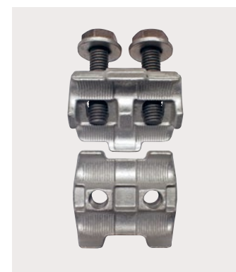
Figure 1: Ideal arrangement of the contact elements. Donati’s rule of current commutation shows that the current density of a connection is not the same at all points: The commutation takes place for the most part at the beginning and at the end of the overlapping surfaces of the conductors. Ergo: The contact areas (zones, lines, points) are placed as close as possible to the beginning or end of the terminal.
