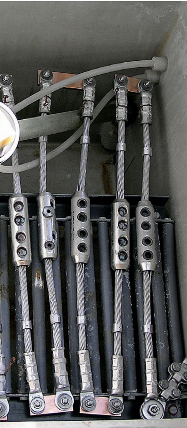
Figure 7: Salt resistance test according to IEC 60068-2-52: The specimens (before cyclic salt spray) are positioned in a test chamber with a volume of 3 m 3 and then sprayed with a salt water solution (5% NaCl). One test cycle lasts 24 hours (2 h of spraying and 22 h of drying). Meanwhile the specimens are subject to cyclic alternating current loads ( I_{on} = 220 A/for 1 h, I_{off} = 0 A/for 2 h).
