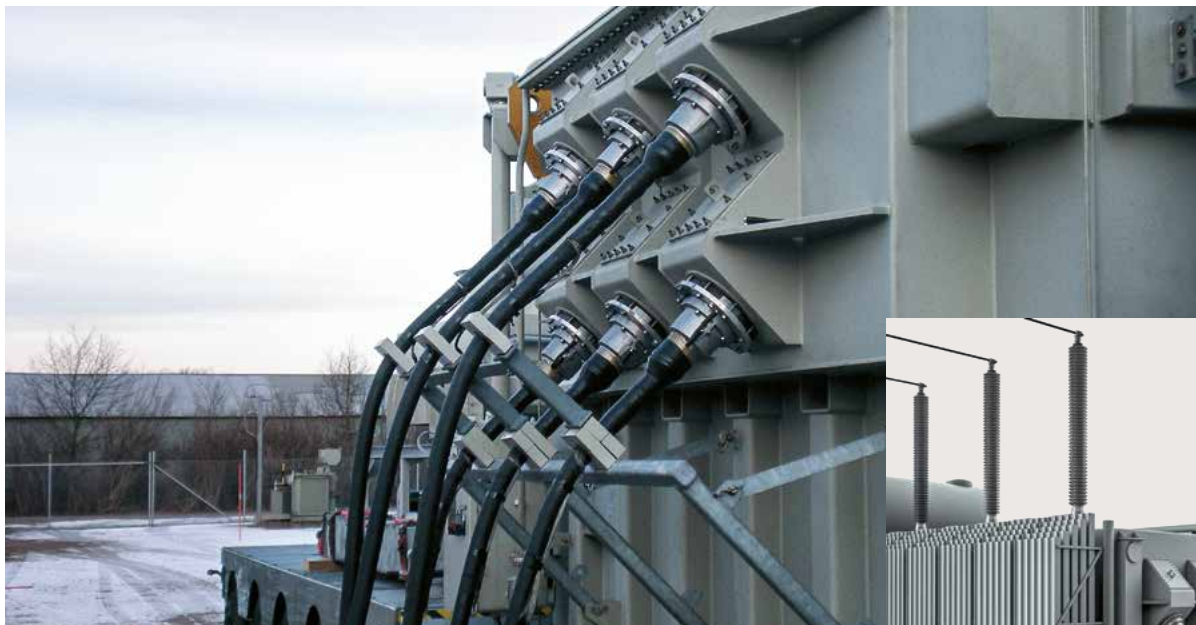
Pluggable HV CONNEX connectors simply plug in during assembly on site. The socket is fitted in the transformer at the factory.
