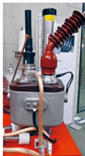
Maximum flexibility: In addition to medium-voltage cables, further CONNEX components are easy to connect to the new MV-CONNEX transformer socket using plug-in technology. Components could include a surge arrester for optimum protection directly at the system (rear right), a test and connecting unit (front right) or an earthing set (front left), as is shown here.
