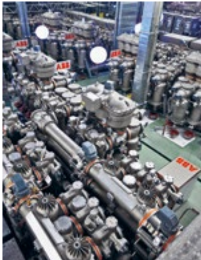
Groundbreaking innovation: The high-voltage switchgear from ABB connects the space-saving design of gas-insulated switchgears with unparalleled low CO 2 equivalent values – thanks to brand new switchgear technology with a patented GIS gas mixture.
