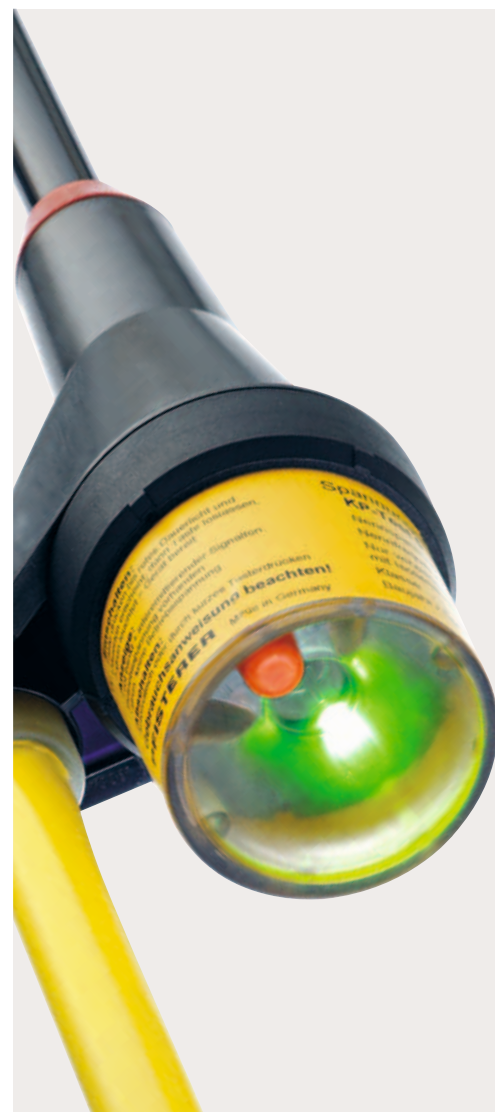
Figure 8: The latest voltage detectors with a built-in active self-test function offer the safest and most user-friendly way of performing a self-test. This image shows a KP-Test 5 model signaling via a lit green LED that a self-test has returned a positive result: the voltage detector is working and ready for operation.
