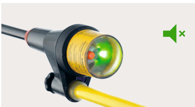
Figure 10: A clear status indicator is a basic requirement for using voltage detectors safely. Their design varies from manufacturer to manufacturer, since the applicable standard specifications leave room for interpretation when it comes to implementing them. Depicted here is a solution which combines visual and acoustic indicator signals as follows: If there is “no operating voltage present,” the KP-Test 5 model shown emits a continuous green light with no beep tone when contact is made with the conductor. However, if there is an “operating voltage present,” six red LEDs flash and an intermittent beep tone sounds.
