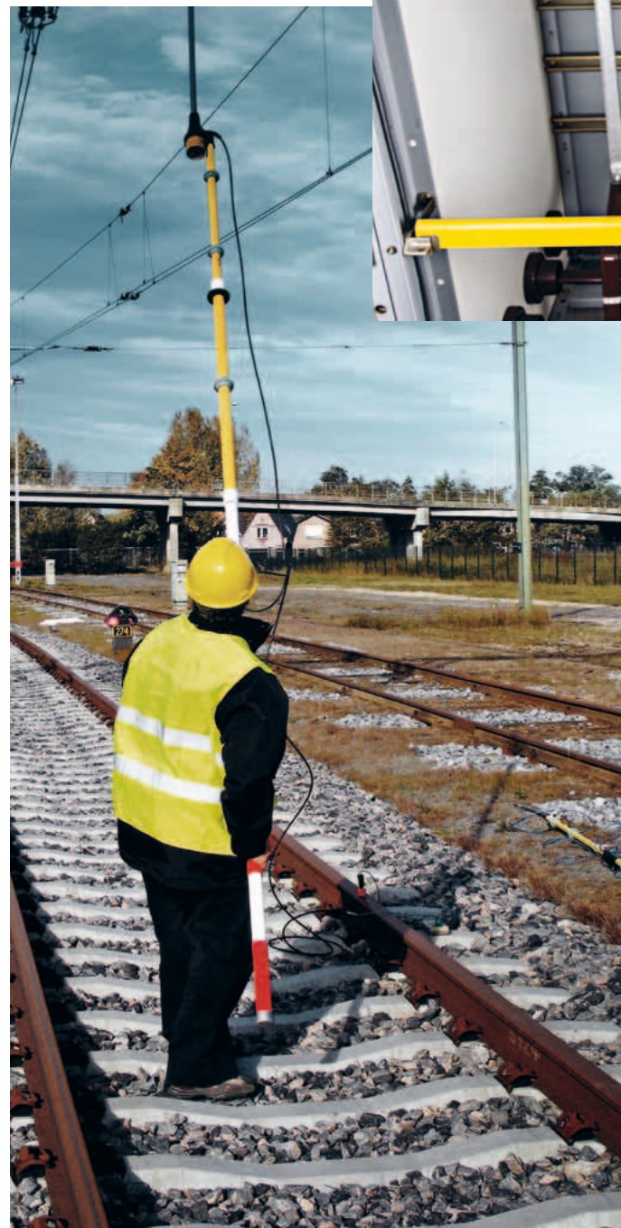
Figure 6 shows a standard instance of two-pole resistive voltage testing in the railroad sector. The voltage detector's second pole is secured to the rail in the form of a magnetic contact.
