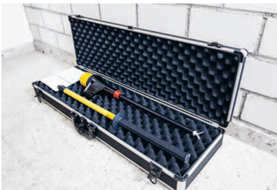
Figure 1: Voltage detector in a special case for transporting it safely to the working place.
