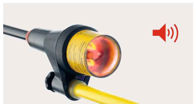
Figure 10: A clear status indicator is a basic requirement for using voltage detectors safely. Their design varies from manufacturer to manufacturer, since the applicable standard specifications leave room for interpretation when it comes to implementing them. Depicted here is a solution which combines visual and acoustic indicator signals as follows: If there is “no operating voltage present,” the KP-Test 5 model shown emits a continuous green light with no beep tone when contact is made with the conductor. However, if there is an “operating voltage present,” six red LEDs flash and an intermittent beep tone sounds.
