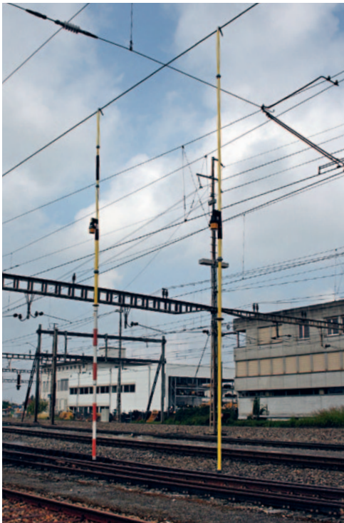
Poor visibility, loud ambient noise? This is no problem for the railway voltage detector, KP-Test 5R: Its visual and acoustic signals are optimally designed for continuously distinct detector readings.
