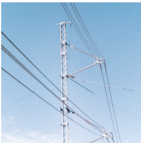
Test set up for the 420-kV insulator crossarm for the Netherlands
