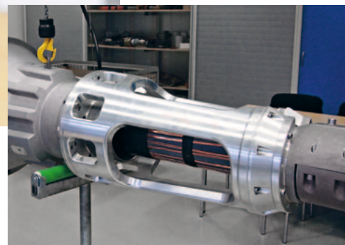
CONNEX connector plug with integrated cable bracing system for constant cable attachment in all installation locations
