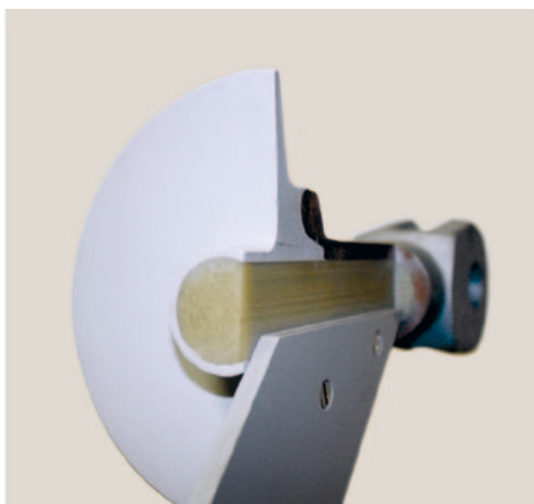
Interior of a silicon composite insulator: Its backbone forms the rod running through the center, which is made of fiber glass reinforced plastic. This must be able to absorb high mechanical forces without breaking.
