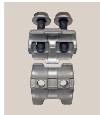
**Figure 1: Ideal arrangement of the contact elements:** Donati's rule of current commutation shows that the current density of a connection is not the same at all points: The commutation takes place for the most part at the beginning and at the end of the overlapping surfaces of the conductors. Ergo: The contact areas (zones, lines, points) are placed as close as possible to the beginning or end of the clamp.
