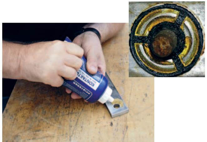
Contact protection paste prevents the oxidation of the points of contact.
