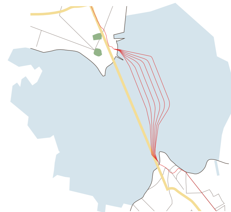
Two three-phase EHV submarine cables are connected to the land cables on both shores using PFISTERER connection joints.
