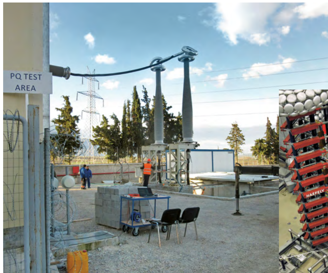
For qualification purposes, PFISTERER's CONNEX and IXOSIL fittings were tested with higher requirements.
