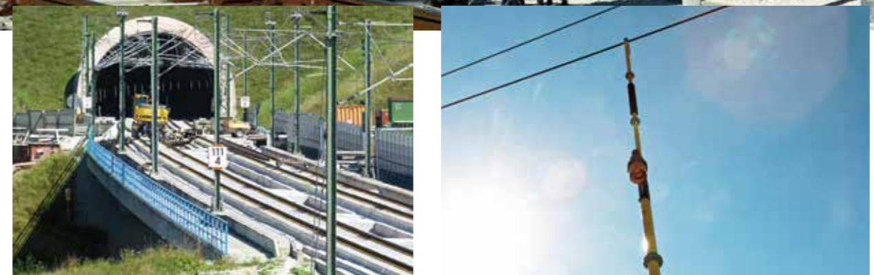
Fig. 2: Adverse environmental conditions: Noise from engineering work or normal railway operations, bright sunlight and other environmental factors can make it difficult to see or hear voltage detector signals. This makes good signal design all the more important.
