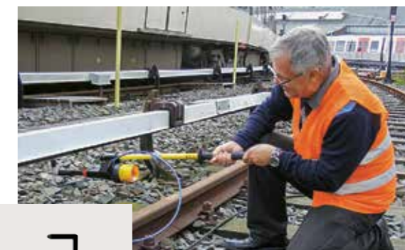
Fig. 7: KP-Test 5 DC for third rail: The test tip extends at 90 degrees on this model variant, so it is easy to make contact with covered power rails on DC railways once the negative pole has been securely attached to the track.
