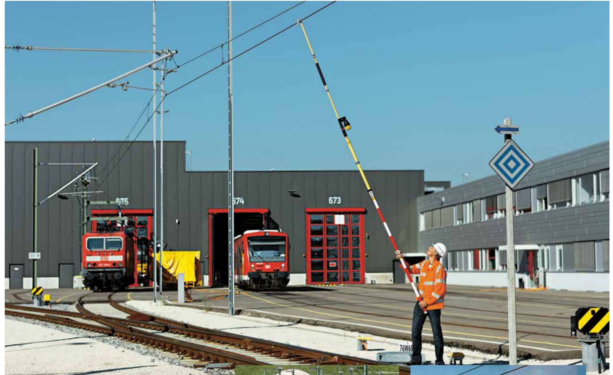
Fig. 1: For railways worldwide: The KP-Test 5R shown in use here is one standard model among many PFISTERER voltage detectors. They are adaptable to fit requirements and enable efficient, safe voltage detecting not only on contact wires but also on third rails, switchgear and power lines.
