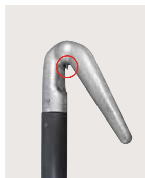
Fig. 5: Making contact the smart way: To make easy and reliable contact, PFISTERER voltage detectors for AC or DC overhead lines have a robust hook electrode. This hooks onto the catenary wire. For optimal contacting, its contact pin (circled in red) penetrates into the catenary wire. Because it is suspended from the wire, the voltage detector's own weight maintains constant contact pressure.
