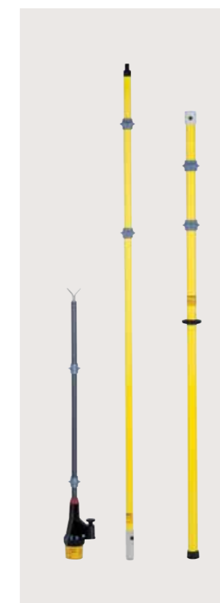
Fig. 9: KP-Test 5H for railway networks: This model is identical in design to the KP-Test 5H for high-voltage applications. It was designed specifically for voltage detection on power supply lines for single-phase railway systems, and has a fork electrode as well as a two-part insulating rod.
