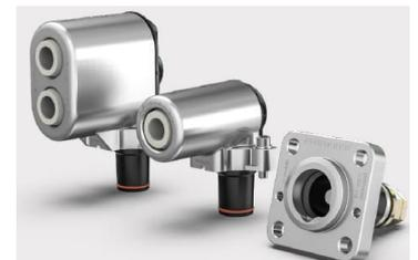
The DNV-GL-certified PLUG MARINE connector system from PFISTERER provides the shipbuilding industry with a robust and reliable contact system for currents up to 1,250 A and voltages up to 3,600 V. The pre-assembled cables with plug connectors significantly reduce the assembly work in the shipyard and during system tests: The electrical connection is established within minutes.
